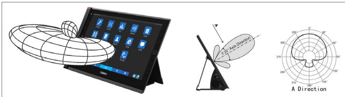
Figure 9 Polar pattern of HCS-8368A/50 Paperless Multimedia Congress Terminal
